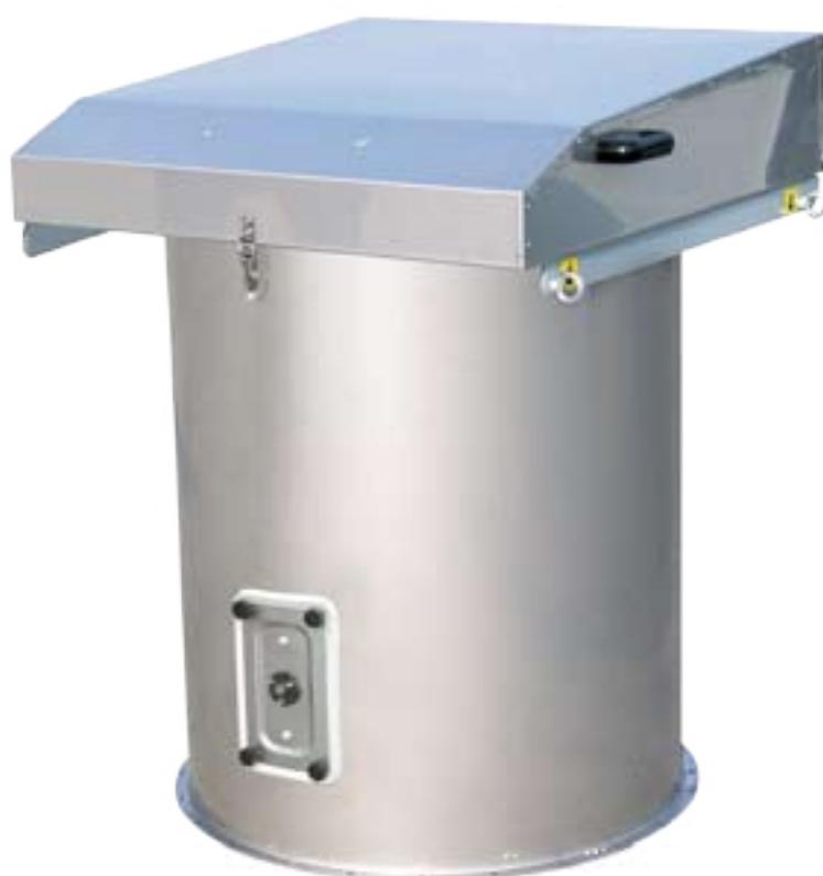
**SILOTOP®** is a cylindrically shaped dust collector for venting of pneumatically filled silos. Dust is separated from the air flow by POLYPLEAT® filter elements and re-introduced into the silo by an integrated automatic compressed air cleaning system. Designed specifically for cement, **SILOTOP®** can be used for all dry non sticky dusts.
