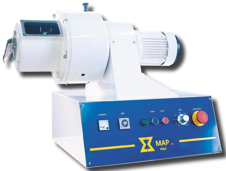
The MLH Laboratory Batch Mixer consists of stand-alone drive unit with incorporated frequency inverter, an easily replaceable horizontal mixing shaft supported at the drive end only, and a quickly removable 180° revolving mixing vessel complete with inlet/outlet.
