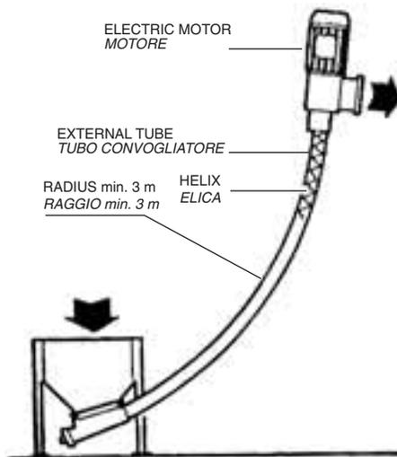
The MULTIFLEX helix-conveyor can be fitted with a mechanical variable speed gear motor.
