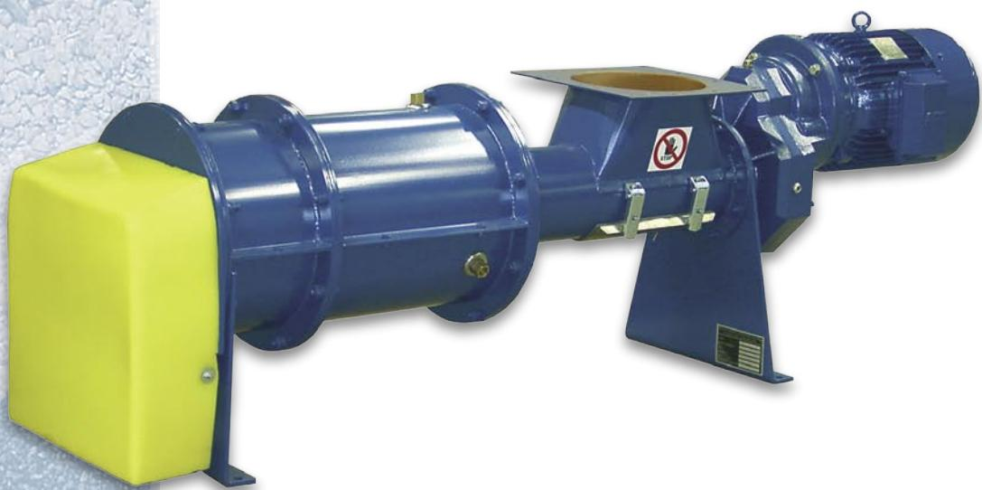
The DUSTFIX® Dust Conditioner consists of a carbon steel tubular casing with SINT® engineering polymer liner, a combined feeder screw/mixing shaft entirely manufactured in SINT® polymer, one vertical inlet and a flush outlet in SINT®, a liquid supply point in the conditioning section, and a drive unit with integrated adjustable shaft sealing unit.
